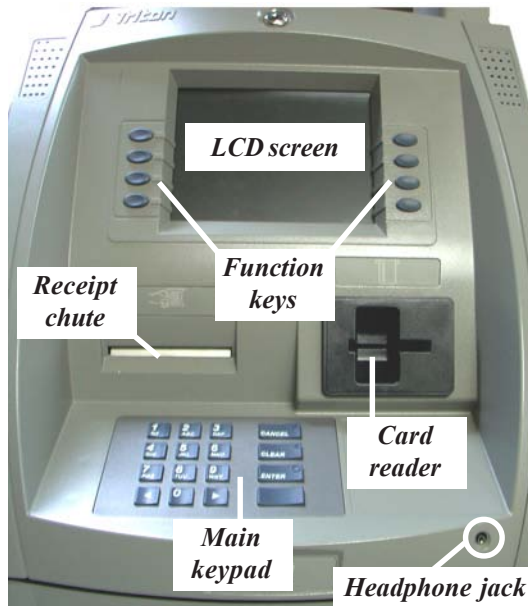
Figure 2-1. Control panel layout.
